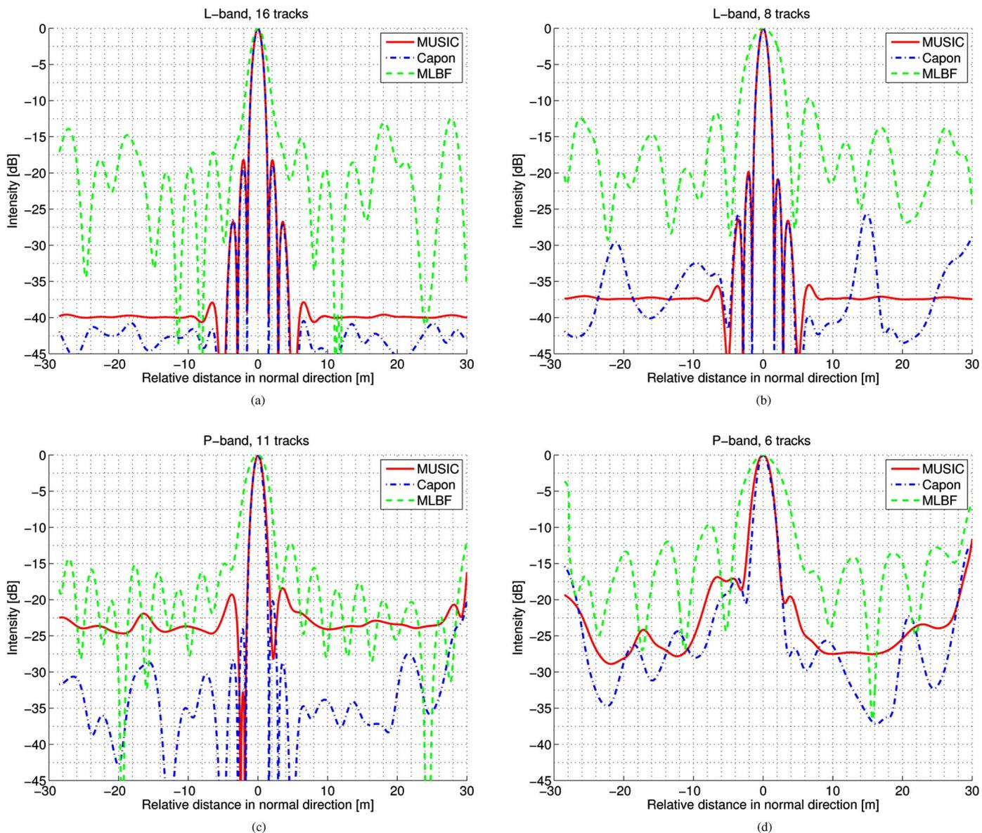
Fig. 2. Impulse responses from a trihedral reflector using three approaches to focus the MB data (HH) in the normal direction: MLBF, RCB, and MUSIC beamforming. (a) L-band, full SA (16 tracks). (b) L-band, reduced SA (eight tracks). (c) P-band, full SA (11 tracks). (d) P-band, reduced SA (six tracks). Twenty looks.
