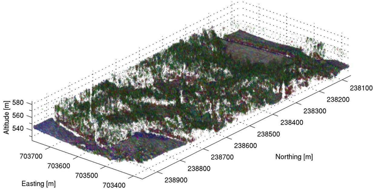
Fig. 3. Tomographic image (3-D voxel plot) of a partially forested area obtained from TDBP-based height-dependent MUSIC beamforming of polarimetric airborne repeat-pass MB SAR data at L-band. Individual scaling. Red (HH), green (HV), and blue (VV). Low intensity = high transparency of the voxel.
