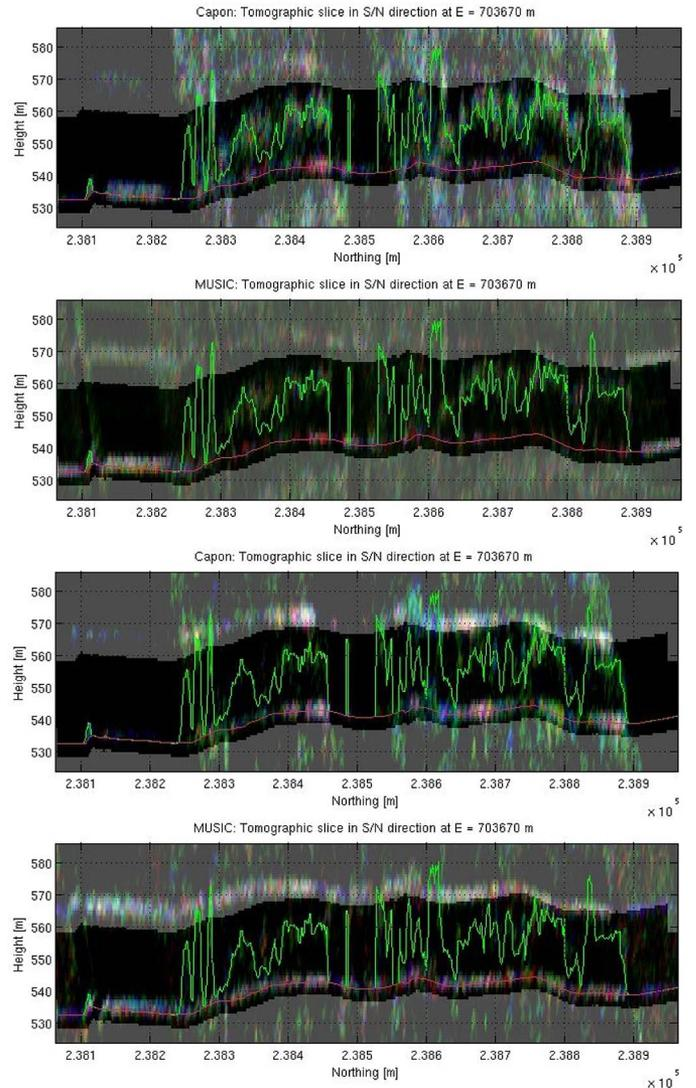
Fig. 4. Vertical slices through a 3-D volume of a forested area obtained from quad-pol MB at L- and P-bands. Red (HH), green (HV), and blue (VV). Individual scaling. (Grayed area) Ambiguous target regions. The tomographic slices run in south-northern direction and are overlaid by the DEM/DSM (solid red/green line) from ALS. Top down: RCB and MUSIC at L- and P-bands, respectively.
