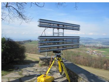
**Figure 1:** KAPRI during the first field test. The top two antennas are the H and V polarized transmitting antennas. The four bottom antennas correspond to the two receiving channels, each with a H and a V polarized antenna.
