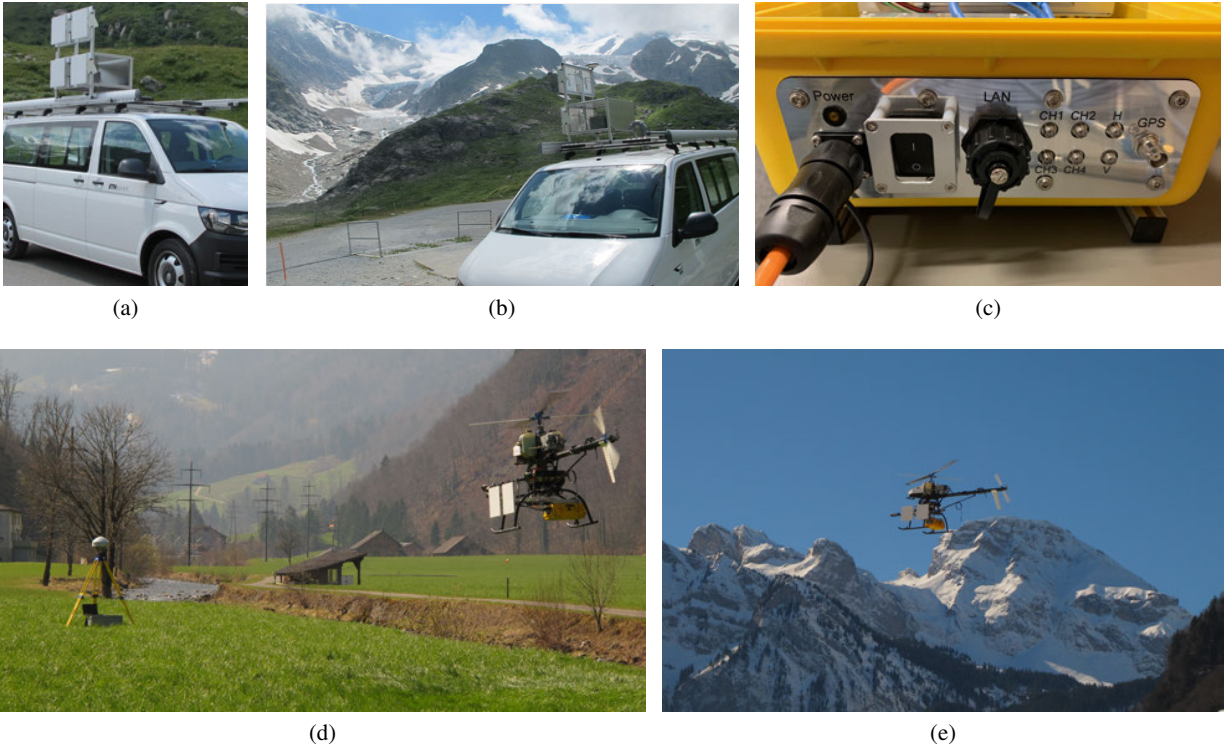
Fig. 1. (a) and (b) : Car-borne setup of the compact FMCW L-band SAR system with one transmit and three receive antennas as used in the Stein glacier demonstration campaign (only one receive channel used here), 2018. (c) Connector plate of the L-band radar with 2 alternating transmit channels and up to 4 simultaneous receive channels. (d) and (e): The L-band SAR mounted on Aeroscout’s UAV Scout B1-100 at take-off (d) and during an interferometric repeat-pass SAR data acquisition (e) in Wolfenschiessen, central Switzerland, in winter 2019.
