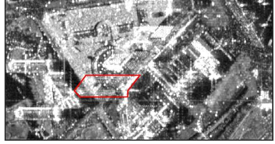
**Fig. 1.** TerraSAR-X average backscatter image of Diagonal Mar, Barcelona, Spain. An example layover-affected building is highlighted in red.
