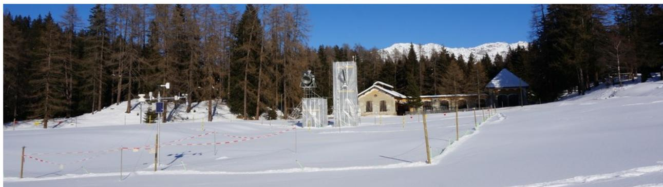
Figure 2: Test site “Laret” in winter 2017. The left tower hosts the radiometers: ELBARA (L-band) and Mora (X-band). The taller tower to the right hosts the rail for SnowScat and WBScat. Direction of the photograph is towards north-east.
