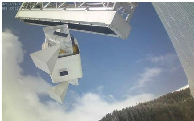
Figure 1: SnowScat is mounted on the tomographic rail that allows a displacement along the rail of about 2.5m. In addition a Quickset pan- tilt-positioner allows to rotate to dedicated angles in elevation and azimuth.
