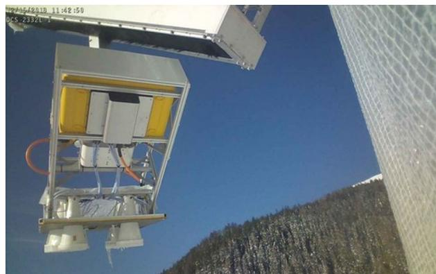
Figure 3: WBScat is mounted on the tomographic rail that allows a displacement along the rail of about 2.5m. In addition a Quickset pan- tilt-positioner allows to rotate to dedicated angles in elevation and azimuth. The yellow box hosts the VNA and controller electronics. At the bottom the 3 pairs of send and receive antennas are visible.
